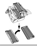
**4** Remove the used film from the cartridge.
